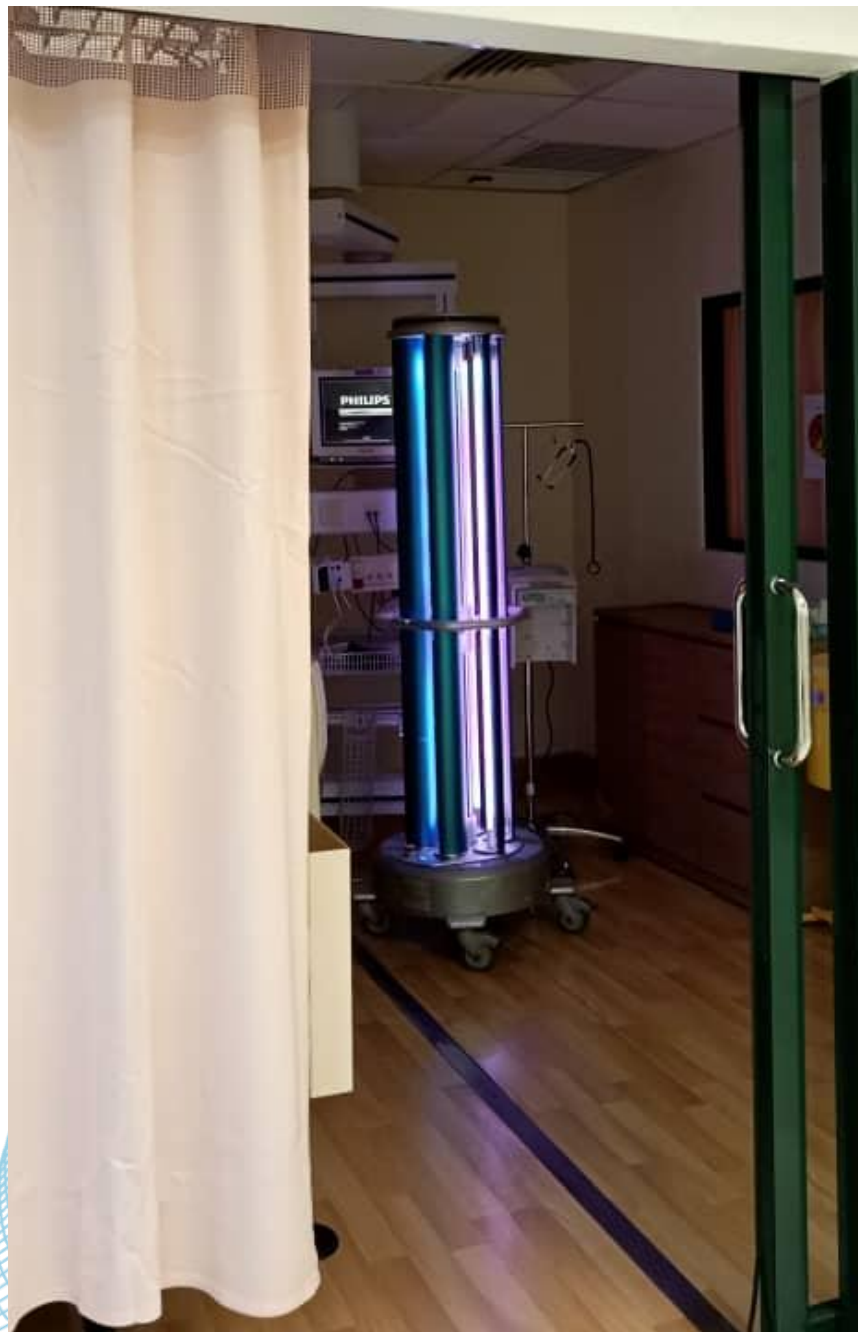
UV light disinfection
